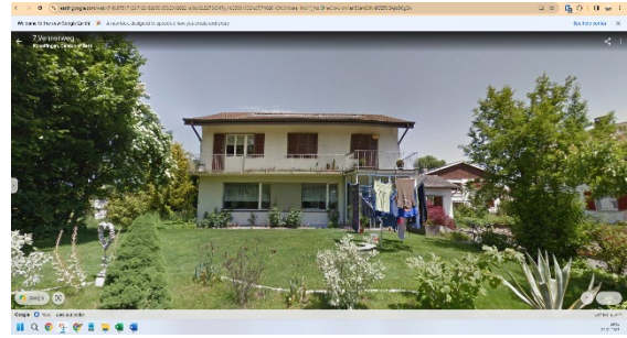
Figure 2: Example building facade with 1 balcony, a summed balcony length of 7 m and a maximum of 2 resp. 3 modules. Source: Google Maps. The potential production calculated for option 1 was 605 kWh/year, 794 kWh/year for option 2 and 908 kWh/year for option 3. Source: Google Street View.
